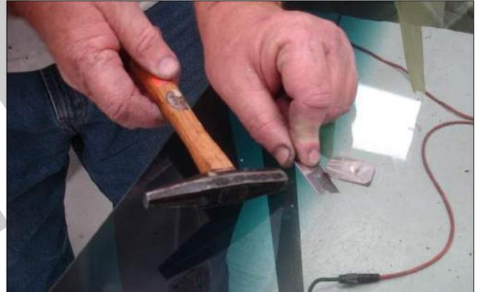
With a quick strike of a small tack hammer the bracket popped off. Looking back it would have been a good idea to wrap the outer (non-striking surfaces) of the hammer head with duct tape or a couple of coats of masking tapes to reduce the chance that I would scratch the glass as I slid it across the surface of the glass to strike the razor.
