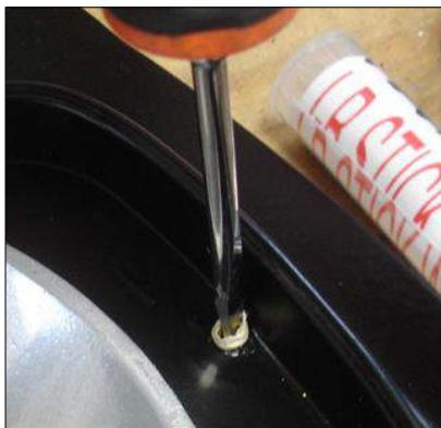
Screw the insert into the panel (it will cut threads during the process, until the bottom of the screwdriver slot is slightly below the surface. Then we used a needle nosed plier to carefully snap off the tabs that stuck up above the surface. Finished results in the picture to the right.
