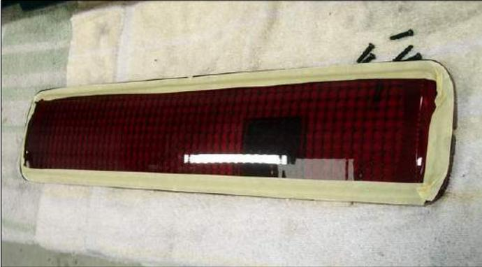
Lens were polished and cleaned then the fronts and rears were masked off to protect them from the paint coat we were going to apply.
