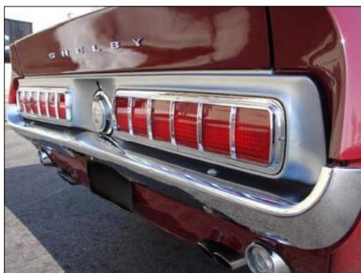
While reassembling the taillight panel I discovered that a number of thread inserts that originally were molded into the taillight panel (to screw the taillight frame screws into) were missing. Unfortunately I did not disassemble the car or I might have found this earlier.
