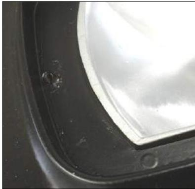
Original threaded insert on right, missing one on the right.
