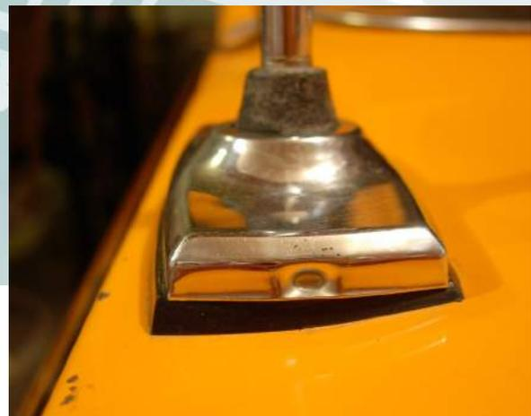
Cougar antenna and gasket installed
