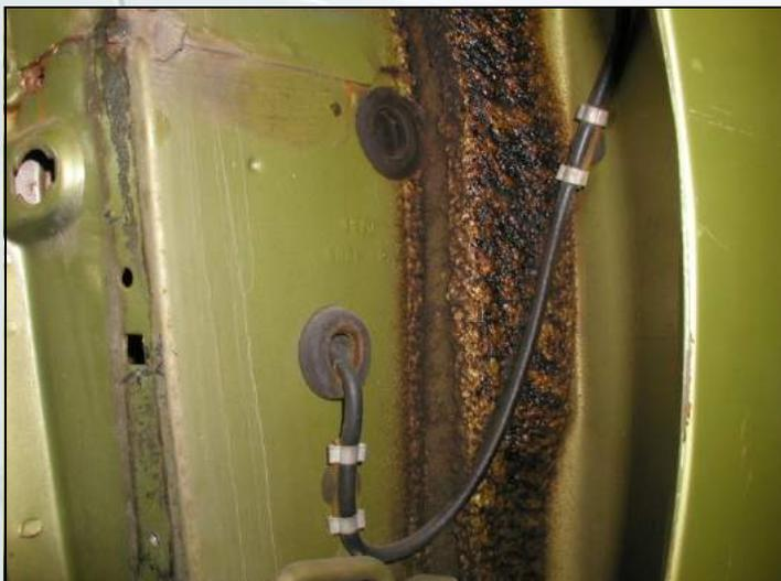
Typical installations and routing of antenna lead from fender thru grommet and into passenger compartment.
