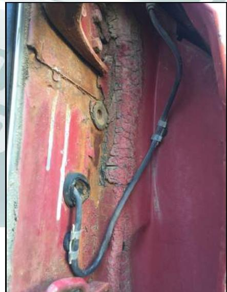
**1969/1970 Shelby Antenna (C9ZZ-18813-C):** The antenna, location, and mounting on the Shelby's was unique because they were installed on the drivers side rear of the car. This was done because the Shelby front fiberglass fenders could not provide the necessary grounding for the antenna and also to solve the problem of interference caused by the ignition system with a fiberglass hood and fenders that was not present on regular production Mustangs with steel fenders and hood.
