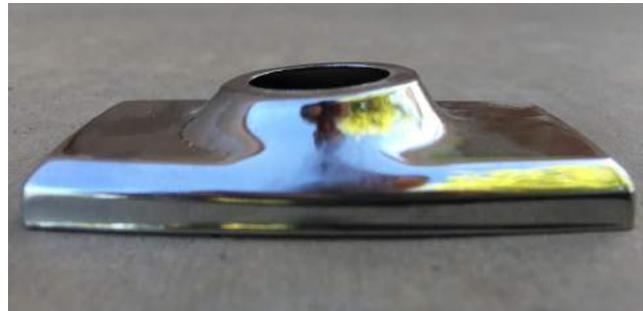
**Original Gaskets—Mustang vs. Cougar** The Mustang had a C9ZA-18898-A engineering number moulded in the gasket and the Cougar was a C9WA-18898-B engineering number moulded in the gasket. This was because of the slight difference in the shape of the fender and antenna.
