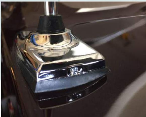
Mustang antenna and gasket installed
