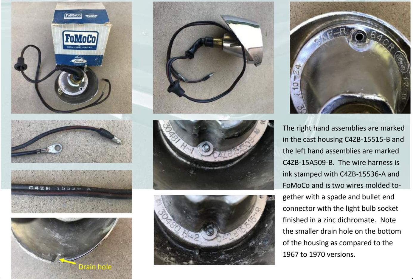
The right hand assemblies are marked in the cast housing C4ZB-15515-B and the left hand assemblies are marked C4ZB-15A509-B. The wire harness is ink stamped with C4ZB-15536-A and FoMoCo and is two wires molded together with a spade and bullet end connector with the light bulb socket finished in a zinc dichromate. Note the smaller drain hole on the bottom of the housing as compared to the 1967 to 1970 versions.
