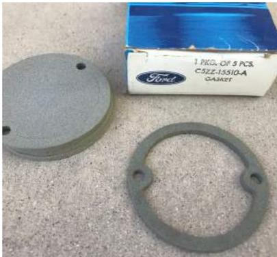
The same back up lens gasket was used all years between the lens (or lenses) and the body of the housing. Shown here these are a grey material C5ZZ-15510-A.
