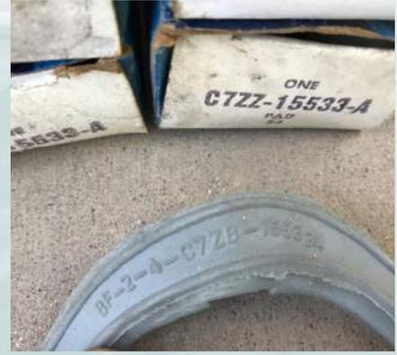
**1967—1970** The second version of back up lamp gaskets were used on all 1967 to 1970 model year Mustangs. Note the correct grey color as assembly line originals had since there is some Ford service replacements that were done in black. The gaskets are now the same for the left and right side and marked with a C7ZB-15533-A, also with a cut out for the drain.
