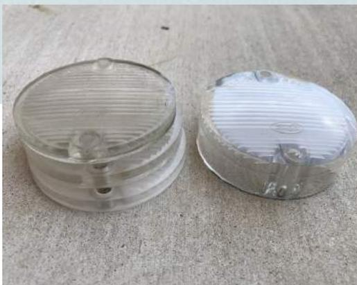
**Left:** Shows the single stacked lenses as compared to the thick lens that was used from April 69.
