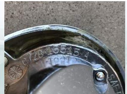
The 1969 and the 1970 model year Ford used exactly the same housing as the 1967/1968 versions, as they are still marked with C7ZB engineering numbers. There was really only two major changes. First was the wiring harness assembly which now has a red connector on the end and the wires are covered in a black polyvinyl chloride insulator and marked with a C92Z-15536-B. The second change is in the design of the reverse lamp lenses which are now marked with a SAE-R 69MG.
