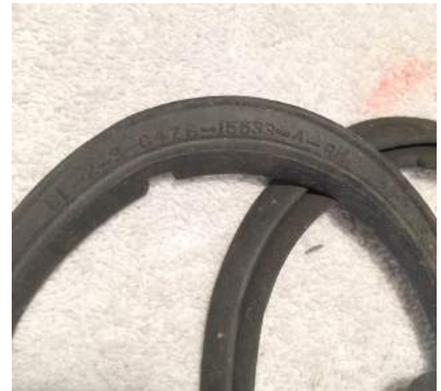
**1965—1966** The first versions of the back up lamp gaskets were used for the 1965-1966 lights. These were originally black in color and were actually separate left and right side gaskets. Left side was marked as a C4ZB-15544-A and the right side was marked as a C4ZB-15533-A with a cut out for the drain hole.
