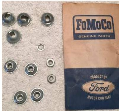
The original mounting hardware shown here that was used for the 1965 and 1966 installations. Besides the mounting nuts, there is a round washer used as well.
