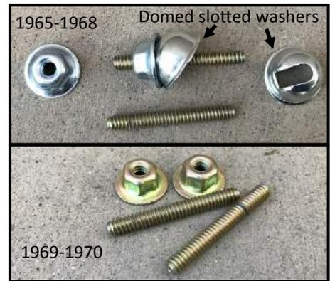
1965 to 1968 applications normally use the domed slotted washer, and 1969 to 1970 does not, even though this washer is still shown in the assembly manual. Unrestored cars (69-70) never seem to have these washers installed.
