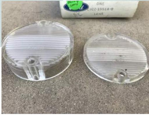
Three different lenses were used from 1965 to 1970. The first lens was used until the end of model year 1968 and is marked with SAE R 64 CR. The second and third lenses are marked the same with SAE R 69 MG with the only difference being the thickness of the lens as described on the previous page.
