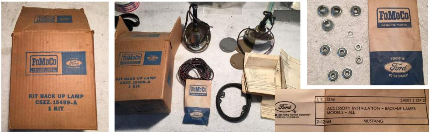
For owners that wanted to add reverse lights on their 1964 1/2 and 1965 Mustangs Ford sold a *Back Up Lamp Kit* under the service part number of C5ZZ-15499-A. This kit included everything from the template to cut the rear valance, to all the wiring, the reverse lamp assemblies, gaskets, screws, lenses etc. Then in 1966 this became standard equipment.
