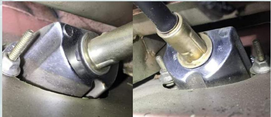
Installation of left and right side of the reverse lights on an unrestored low mileage 1968 Mustang. Shown here is what is typical for the hardware and note the distinct L and R for the right and left side assemblies that can be seen once the lights are installed.
