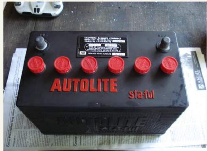
**The first step** is to discharge the battery as much as possible. I connected an old tail light to the battery with temporary leads and let the bulb burn around the clock. It took several days for this one to go "dead". Be careful about the surroundings during this phase as the bulb can get hot and you don't want to return to something melted or burning.
