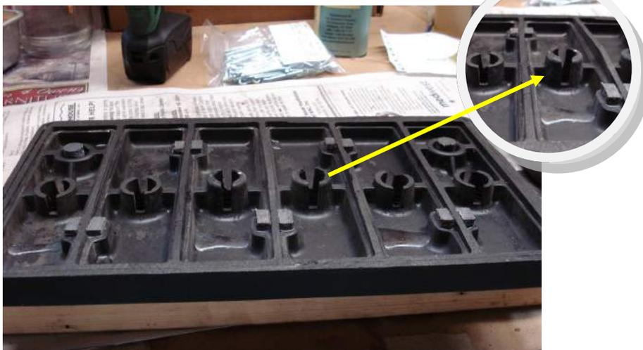
Here is the other tedious step in this process. You need to drill and tap a hole in the underside of the lead posts for a threaded stud. The word of caution here is that the lead is tricky to drill because the swarf tends to fill the flutes on the drill and can abruptly bind the drill bit in the hole. Don't even think about drilling a small pilot hole first, because this increases the risk that you will break off a drill bit if/when it binds.
