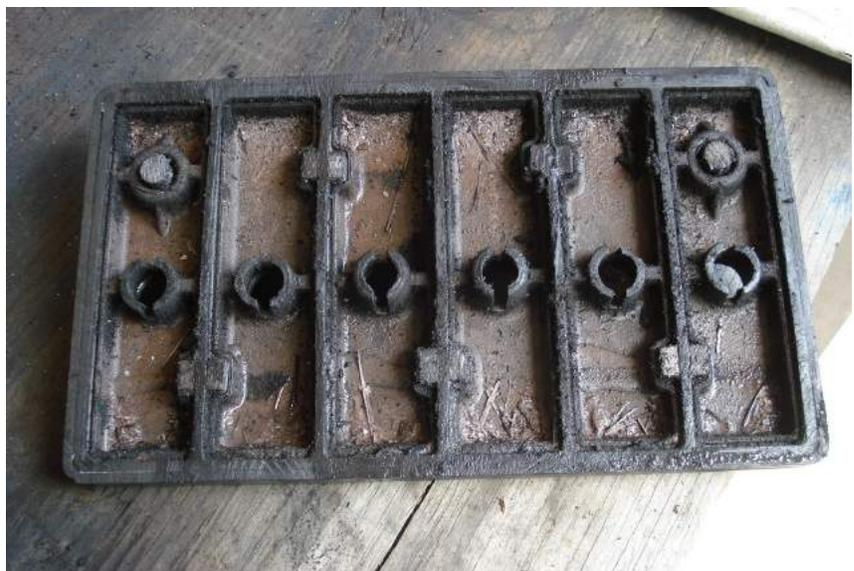
As you can see, there are two posts and five pairs of lead bars that must be separated with the saw. I also cut through a portion of some of the filler cap nipples, though this is not necessary in order to separate the lid from the case and represents extra work at this stage.
