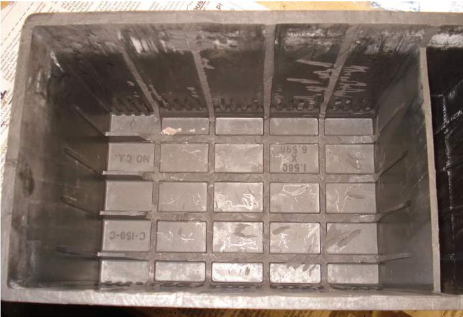
I mentioned that you do not need to remove the fill cap nipples to remove the lid, but you may need to trim them down for battery clearance. I went ahead and cut the nipples off flush with the cut I had made to remove the lid. In these pictures, there are still two nipples that need to be trimmed. The cutoff wheel works great for this.
