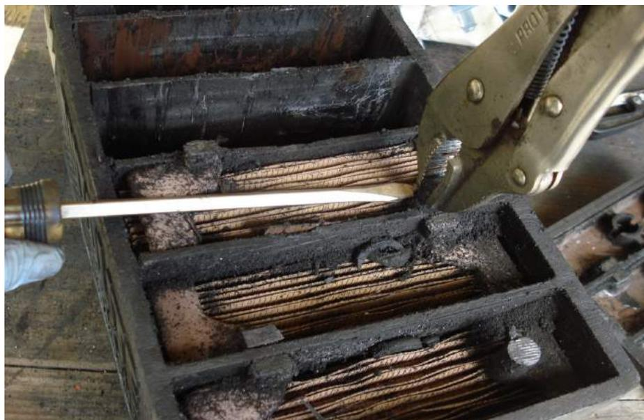
I placed the plates in a plastic bag for disposal. My local battery distributor will accept these plates and the bottle of acid at no charge and I assume they recycle the plates and safely dispose of the acid.
