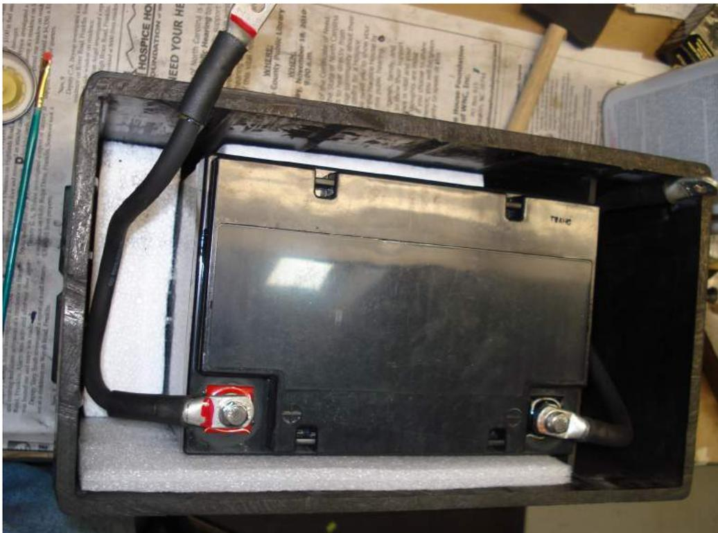
Note that I trimmed the remaining case partition with the cutoff wheel to make it level with the case of the new battery. This is necessary so that there is clearance to route the cable. I also used some scrap styrofoam to fill the gaps between the new battery and the case so that it wouldn't slide around or rattle. I didn't bother with padding the top as I didn't want to interfere with the fit of the lid and I thought the chances of the new battery hopping up and down in the case was slim.
