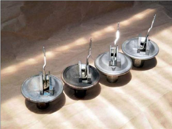
The four test diaphragms. For reference, I marked the control arms with a felt tip: all permanent markings are on the distributor side
