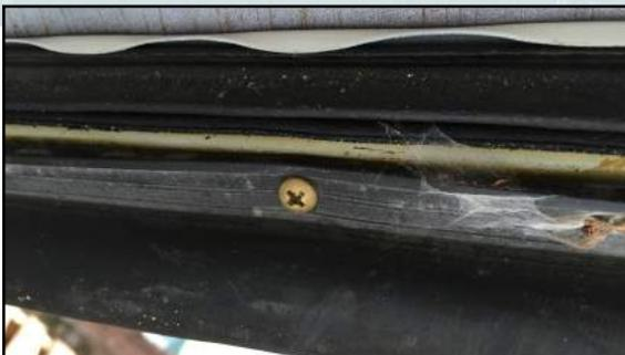
**Original Mounting Hardware:** The original mounting hardware that should have been used was specified as a 383379-S100 screw and washer in the assembly manual. Although this should have been used, other type screws were used as well as shown here. Typical finish seems to have been a zinc dichromate as pictured here on this original low mileage Boss429 on the left.
