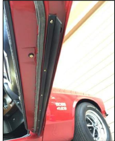
One of the most common missing parts on a 1969 Mustang or Cougar today is the lower weatherstrip seals on the doors. These seals were added to cars to keep dirt and moisture from entering but usually are missing or damaged even on original low mileage cars today. And because most people do not realize they are missing they are usually not put back on during the restoration process. This quick guide here will show some examples and the correct installation and mounting hardware for the seals.
