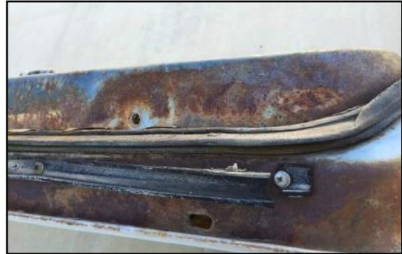
This shows what's typically what's left on a car if it still has any of the door seal and the mounting hardware in place. The channel of the seal is still in place but the sweep is long been torn off or fell off.
