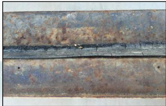
Many original doors still have the pilot holes visible where the seal would have been installed. Shown here is Bob Perkins original 1969 50 mile Mach 1 on the left and a 1970 door on the right. Note how small the pilot holes are.
