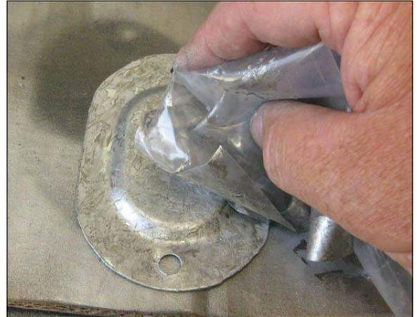
bright base zinc will show through providing another level. The finished look should have about 40% of the bright zinc showing through (partially or fully in places) while the other two shades make up the balance.
