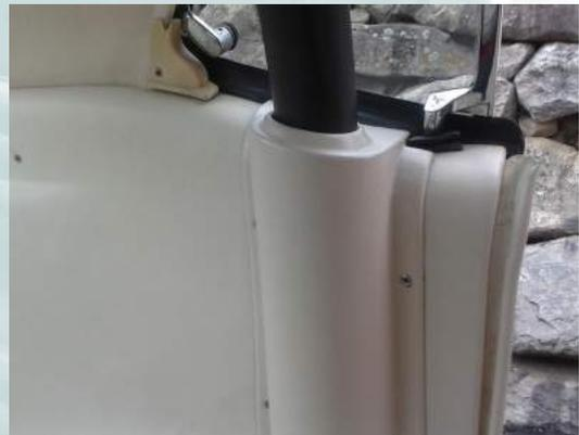
The 1969 and 1970 Shelby interiors came in only black and white so these panels only come in two colors. Because of the cut out area for the roll bar you see these pieces being different than a normal fastback piece. All Shelybs should have the quarter window cap.
