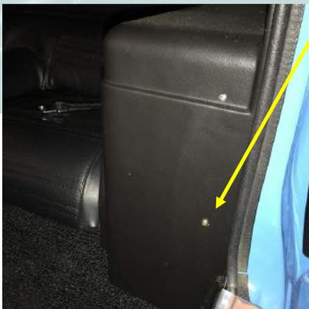
**Gold?** It is not uncommon to see on original cars the lower panel screw being different and actually being a zinc dichromate finish. This would be instead of the silver finish we see on the other screws for this panel.
