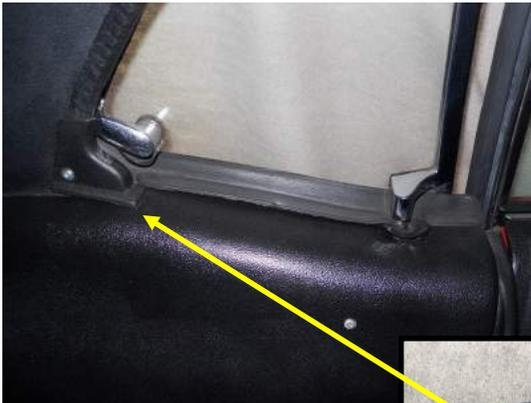
**1969** Shown here with the quarter window cap to cover the cut area of the panel. This piece is not used on a 1970.
