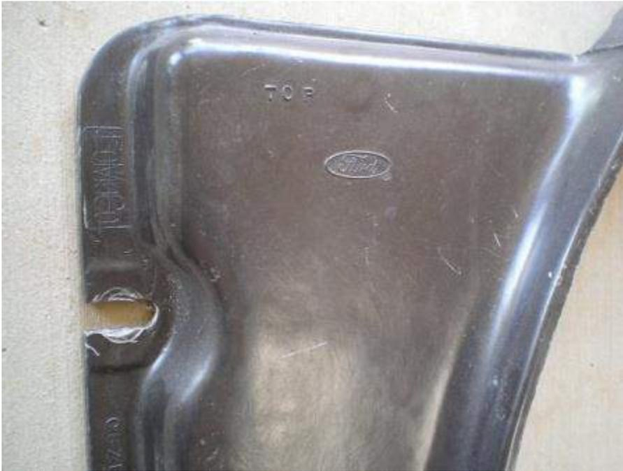
Fan shrouds with a lined out FoMoCo on the side are considered service replacements as they would not have appeared in regular assembly line cars, except possibly on some of the last built 1970 Cobra Jets.
