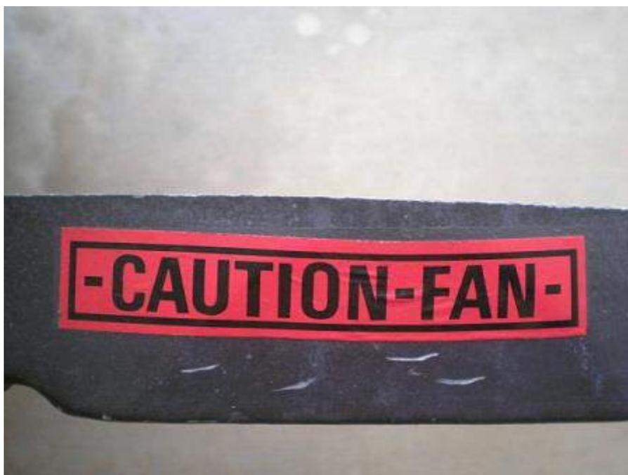
One important note: The only fan shrouds that ever came with a "Caution Fan" sticker were the service replacements. This may have started in the mid-1970s. This sticker was not placed on the fan shroud for factory assembly during the 1968 to 1970 model years. There have been discussions that they may have been placed on cars by the dealer when the vehicle came in for service at a later date, possibly related to a service bulletin.
