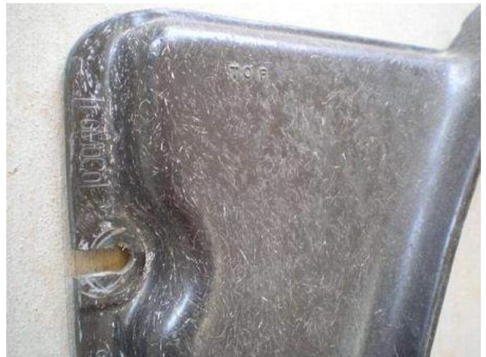
The C8ZE-8146-A version was the original design shroud and would have been installed on the 1968 428 equipped cars. It is simply identified with the word TOP molded in the top left and the edge molded with a large square FoMoCo logo, C8ZE-8146-A, and Barnum Bros. Fibre Co., Inc.
