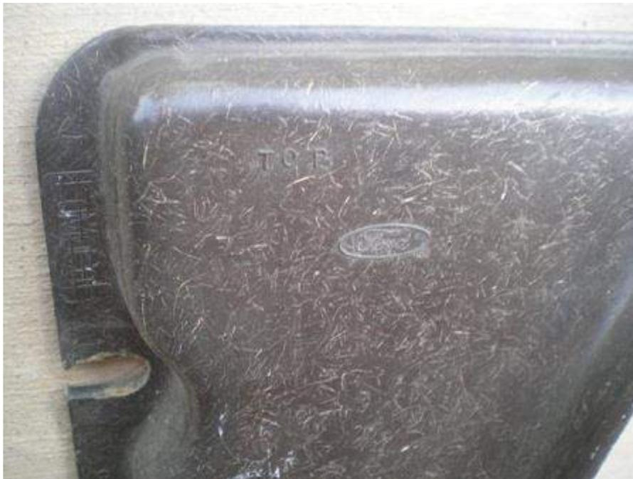
The third/service version, which is the service replacement which was sold at Ford dealerships up into the 1990s, has the oval Ford logo in the top left and the word TOP. The edge is molded with a large FoMoCo that is lined out, C8ZE-8146-C, and Barnum Bros. Fibre Co., Inc. The texture of the fiberglass on these fan shrouds now is a smooth texture with no glass fibres visible anymore and the shroud feels slightly more flexible.
