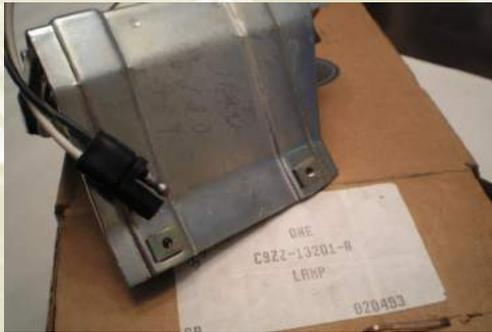
*In the mid 70's Ford started selling the 69 turn signals with two pin wire plugs. It is hard to imagine Ford making that mistake, but they are incorrect. They do not fit/mate with the existing wiring on a 69 Mustang. They are still sometimes found NOS today—**Buyer Beware.***
