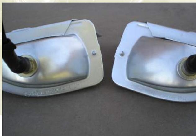
Original 70 housings where you can see the contrast between the two different finishes of the socket and housing.
