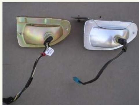
Between the two years the metal housing assemblies are completely different, with the three main differences being the attaching bracket, the wire harness, and the finish.
