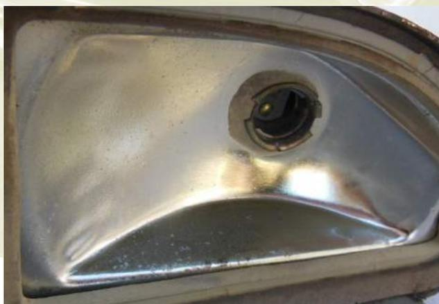
Sometimes you can still see the round area left with no paint at the opening for the bulb holder, which assured proper grounding.
