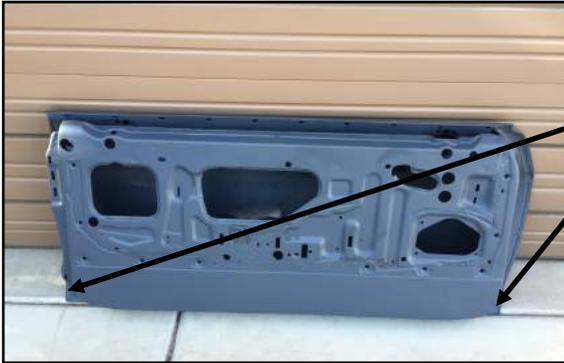
Shown here for reference the areas on the inside of the door that differ between 1969 and 1970. This would be the two inside corners of the door –on both the front and rear edge of the door.
