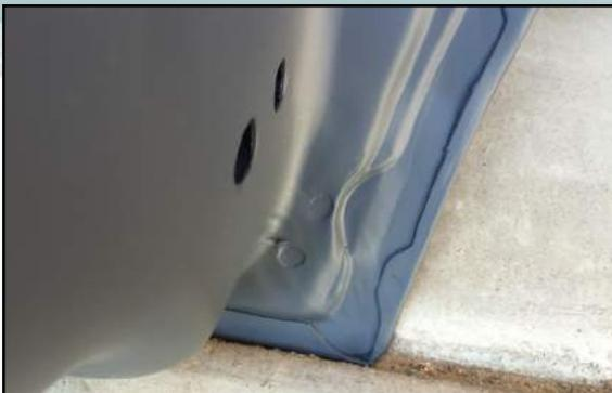
Shown here the added recessed areas that don't exist on the 1969 doors with the installed mounting hardware for the Mach 1 trim.
