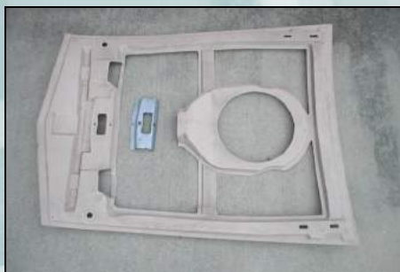
Original support structure from the underside of the Shelby hood
