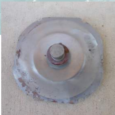
The steel diaphragm
