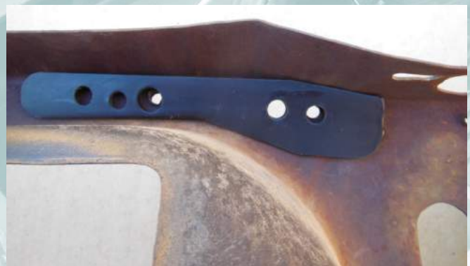
1970 radiator support to show clearance issues.
