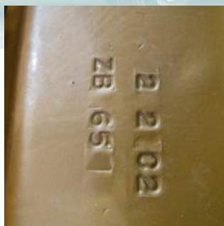
**Date Codes:** Visible on the underside, and unlike the fastback trunk lids, are not reverse stamped. The format shown would be month, day, stamping plant and shift. The ZB 65 refers to the body style.
