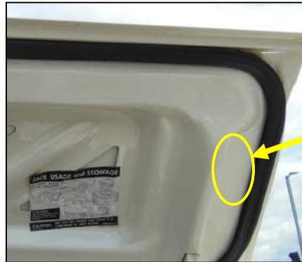
The main identification on a 1969 trunk lid is the lack of a cut out in the underside seen in the circled area.
