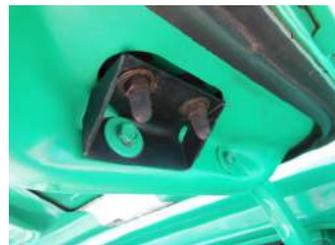
Original paint rear spoiler mounting with 1970 bracket shown. Notice the hinge bolts would be painted and only the bolt that was removed for the spoiler bracket would be chipped.
