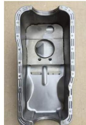
**The basics:** To show the difference inside the oil pan, with and without a baffle, the pictures here show a regular production 1970 302 oil pan, versus the 1970 Boss 302 oil pan with the baffle installed.
