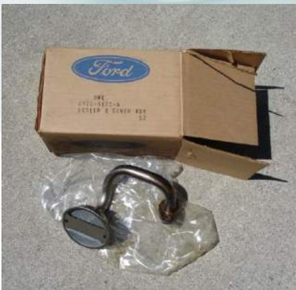
The Boss oil pans also used a special oil pump pick up that is shown here. This was the C9ZZ-6622-A.
