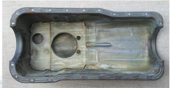
**1970 Version D0ZZ-6675-A:** This version of the oil pan is the same as the 1969 version with the exception of the recessed areas in the bottom of the oil pan itself. Most likely this was done to give additional clearance for suspension.
