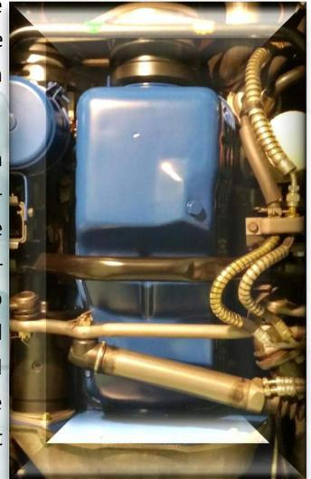
For 1969 and 1970 Ford used two different styles of oil pans for the Boss 302 motors. The 1969 oil pan is the standard C5 289 oil pan that has been modified to add the baffle inside. The actual part number for the oil pan with the baffle makes it a C9ZZ-6675-C.
