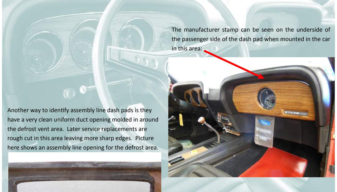
The manufacturer stamp can be seen on the underside of the passenger side of the dash pad when mounted in the car in this area:
