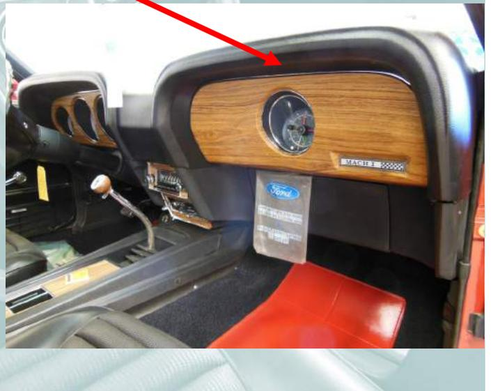
Another way to identify assembly line dash pads is they have a very clean uniform duct opening molded in around the defrost vent area. Later service replacements are rough cut in this area leaving more sharp edges. Picture here shows an assembly line opening for the defrost area.
