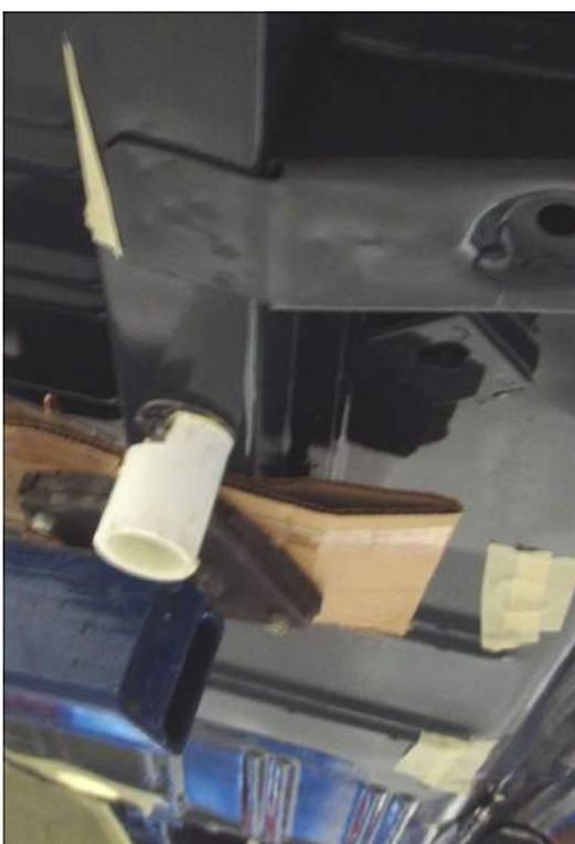
An earlier design had a cut out in the side of the tube to allow me to hold the nut while I tightened the bolt (single sided tool). As I discovered, gluing the nut to the tube and washers allowed me to do away with this extra work.
