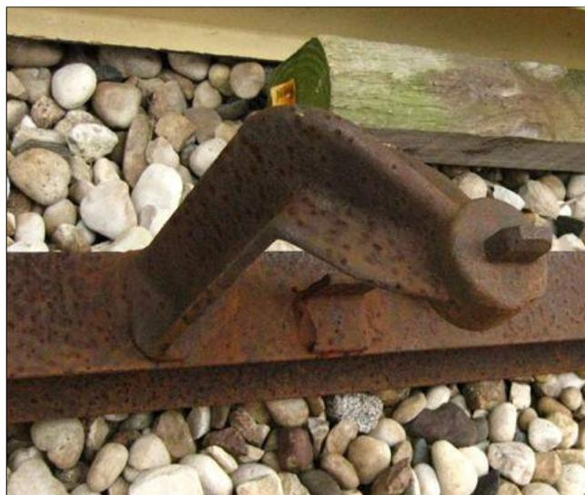
Here is a close up of the rear mounting stands (in this example from 69-70—see last page for explanation) . At this point (and one further forward) the car was bolted to the dolly.
