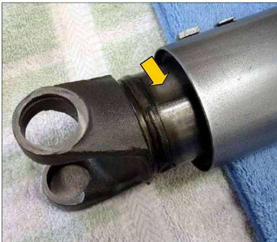
This driveline happened to be of the tube-in-a-tube design so I could not forget the heat seam on the inner tube.
