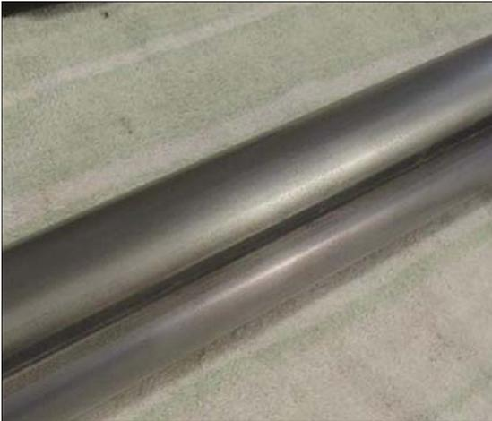
Finally I removed the last of the tape and lightly sanded the heat stripe and the edges so that all noticeable signs of the tape (sharp edges) were erased and the overall look was muted. Once you get a good consistency (one end to the other) stop!
