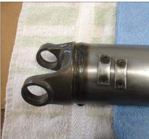
Using the gun bluing solution and a brush I spread the liquid over the welds found on each end of the tube.
