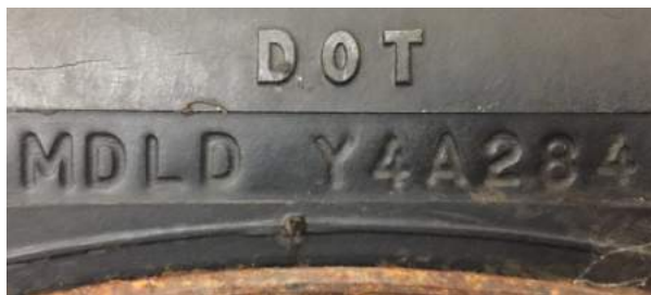
MDLD Y4A284—last three digits indicate 28th week of 1974
