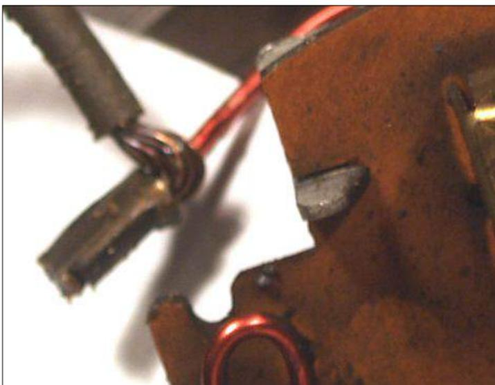
The original connection from the input cable to the armature winding wire was made with a crimp. I used my Dremel tool to cut the crimp off as I wanted the extra length (3/8 inch) of the coil winding wire.". It's a bit tight in there.
