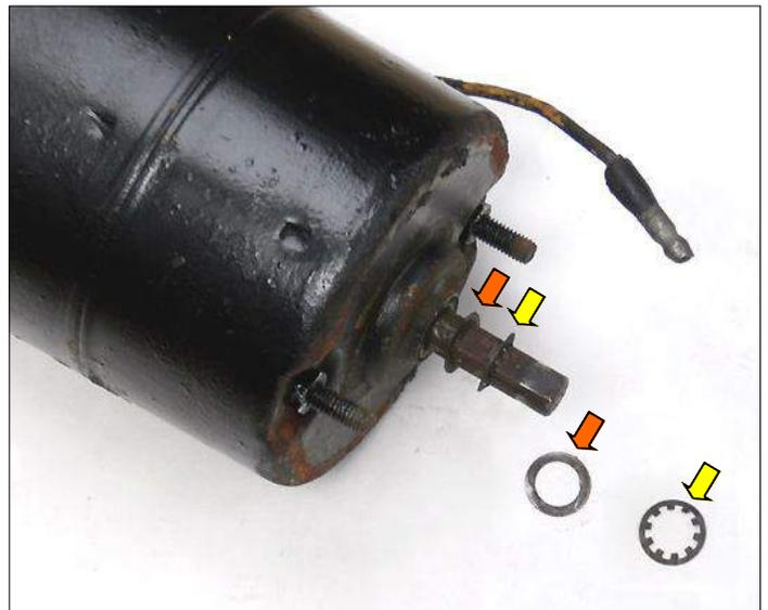
The picture above shows a motor with the retainer and washer slid down the shaft and another retainer and washer for size reference.
