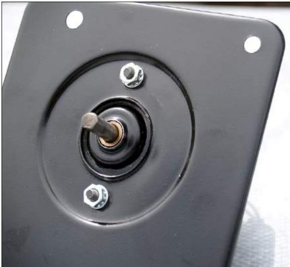
Install the mounting plate on the two long screws over the seal. Note the offset left hole and the plate edges turned away (towards the engine compartment). Not shown is the wiring grommet and leads located on the top when the motor is installed properly.
