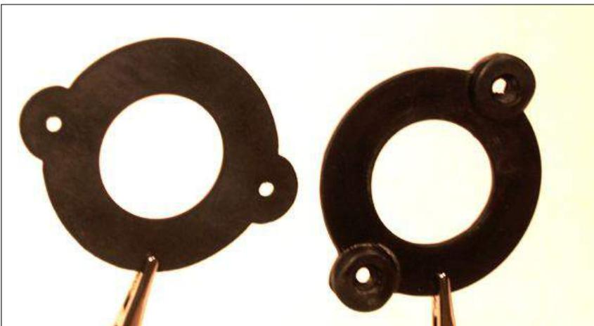
The seal in the heater rebuild kit is a flat piece of rubber, shown on the left. The factory seal, on the right, has bumps that fit over the two nuts on the long housing screws. I reused a good factory seal.
