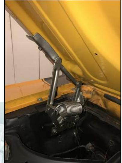
The original style hood hinges that were used on Mustangs, Shelby's, and Cougars between 1964 1/2 and 1970 are similar, and in some cases interchangeable. This guide will help identify the differences and show the details to look for on factory original hinges and springs. The hood hinges came in three basic designs during those years as listed below. The hood hinge springs came in four different styles also listed below.
