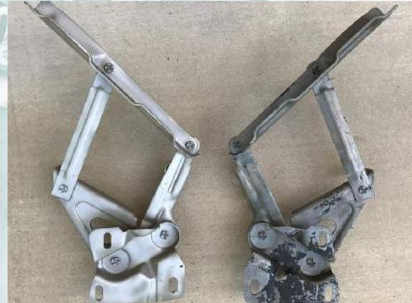
**1969-1970:** The third generation of hood hinges, the C9ZZ version has a completely different arm for extra hood to hinge clearance that was needed. The X rivet design was used until early 1970 production when the dished version rivet started to appear and was used for all service replacements after that. Most originals have date codes.
