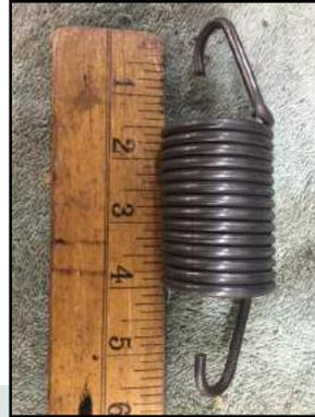
Special Shelby spring S1MS-16796-A was commonly used on cars that had fiberglass hoods (both sides) or cars that had steel frame with fiberglass hoods (on one side only). Overall length is about 5 1/2 inches.
