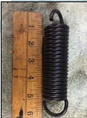
Special Shelby spring S7MS-16796-B was commonly used on 1967 Shelby (all fiberglass hood cars). Overall length is about 6 inches
