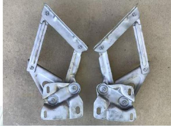
**1967-1968:** Second generation of hood hinges, the 1967/1968 version was used until 1968. Change over date from the C7 version to the C9 version started around March of 1968. During that time you can find some cars with both version hood hinges on the same car. After that, eventually all service parts were the C9ZZ version (below) as they are interchangeable. Originals have X rivets and most have date codes.
