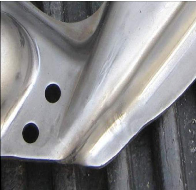
This article focuses on the refinishing of tie rods but the process and techniques can be applied to many of the suspension parts used on classic Mustangs and Shelby's. Though the article uses gun bluing repair fluid and/or paste, an alternative to this is using a quick manganese phosphate dip of about 30 seconds.
