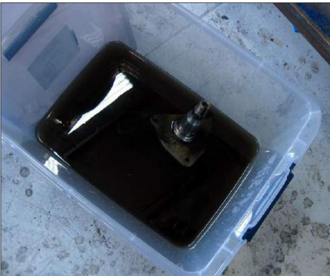
First task is to clean the parts of all the old oil, grime and any surface rust. If the metal is damaged from pitting you will need to find a replacement in better condition. Also inspect for any heavy damage from parking curbs or from their removal. Light damage can sometimes be removed by dressing the area with a file but you will have to evaluate each piece for its acceptability.
