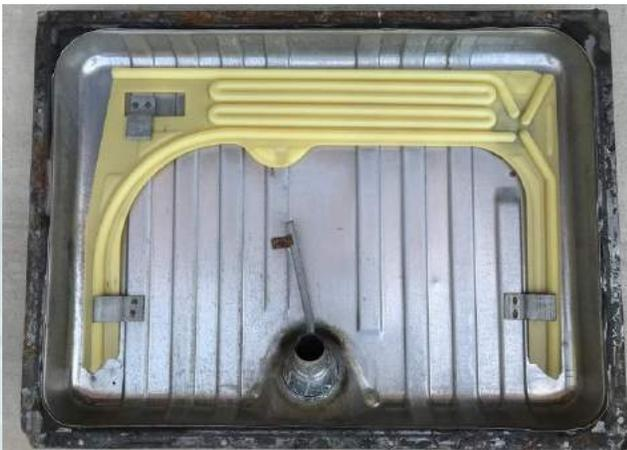
Shown here is the special CA fuel tank completely split open to show the internals showing the top half view. Note the extra tubing that is used to recover the fuel vapors. It is because of all these extra parts its impossible to clean out and reseal one of these tanks.
