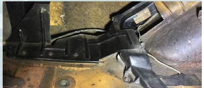
Both Mustangs and Cougars use the same exact bracket to hold the front and rear fuel tank vent expansion units. Part number for this was a D0ZZ-9A188-A and would be painted black and installed after the car was painted so it should not have any body color on it to be correct. Self tapping screws were used to hold the bracket in place (usually zinc dichromate).
