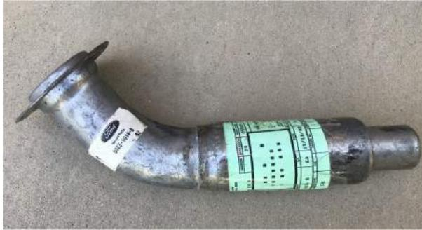
Shown here an NOS Mustang filler neck marked with the DOZZ-9034-B part number. Note different design when compared to the normal filler necks and the correct tin lead finish which does not corrode to fuel.
