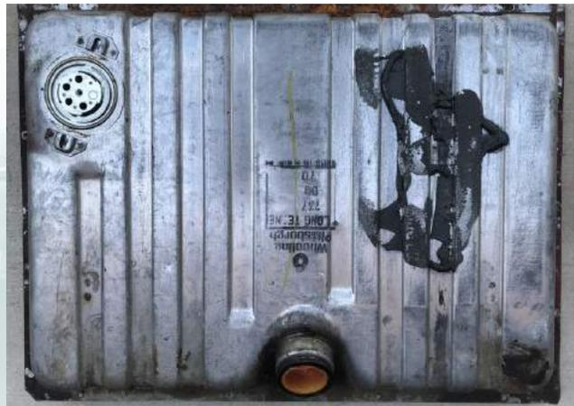
It appears that almost all of the CA emission fuel tanks were manufactured by Wheeling Pittsburgh as indicated by the stamps that are seen on surviving cars and fuel tanks. Note also the grey sealer used to hold the anti rattle board in place on top of the tank.
