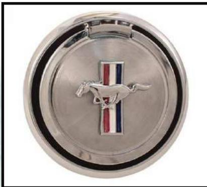
D0ZZ-9030-D pop off style cap that was used with the 1970 Mach 1 package also had the longer neck to accommodate the CA emissions package.
