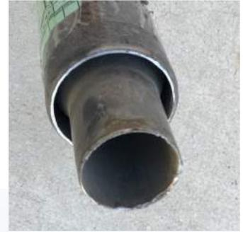
The unique end of the filler neck on these units when compared to a vented system.
