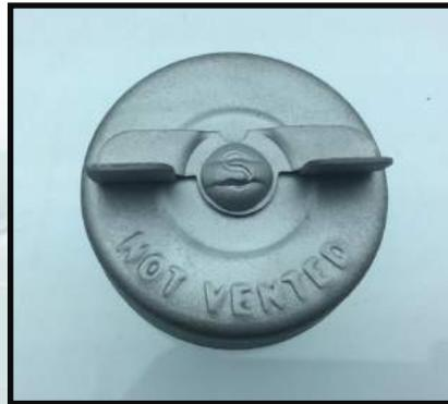
D0AZ-9030-A style cap non vented, used on Cougars. Note the S stamped in the center rivet which is the manufacturer stamp for Stant.
