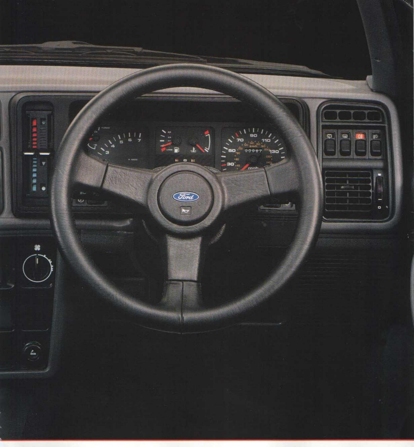
lights are clearly visible through the padded, sports-type steering wheel. Minor controls include a quartet of micro switches to the right of the wheel, and, to the left, smooth-sliding levers for the sophisticated heating and ventilation system. Ford's applied ergonomics make everything easy to see, identify and operate.
