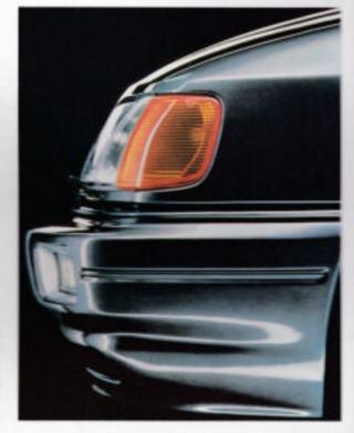
bumper is filled with a special plastic foam to resist low-speed impacts. Its lower lip is shaped to smooth airflow past the wide-rim alloy wheels.
