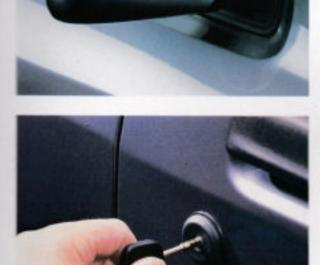
Electric motors enable the bodycolour door mirrors to be adjusted with pin-sharp precision at the touch of a button. They are also heated, to maintain rearward visibility when the temperature drops below freezing point.
