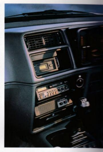
The illuminated graphic display module warns of bulb failures, doors that have not been fully closed, and low ambient temperatures.
