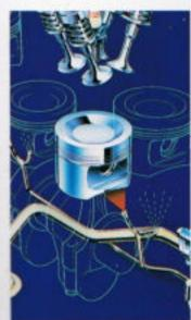
an extremely efficient combustion chamber whose benefits include good fuel economy† and low exhaust emissions. In addition, the volume of gas that can flow through pairs of inlet and exhaust valves is about 50 per cent greater than the figure for the biggest single valves that could be fitted to a combustion chamber of the same size. Increased gas flow is synonymous with increased power.
