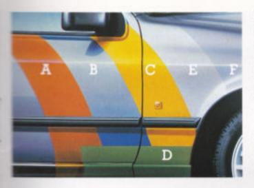
The quality of Ford's multi-stage paint and protection treatment is endorsed by a six-year anti-corrosion assurance. Critical box sections and other areas are injected with wax. Plastic liners provide extra protection for all four wheel arches. High-quality aluminised steels are used in the long-life exhaust system, to combat internal and external corrosion.
