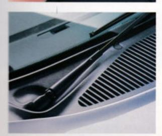
Wind tunnel tests emphasised the value of semi-concealed wipers. They are fitted with small, blade-like aerofoils shaped to keep the wiper in contact with the glass at high speeds. The screen itself is electrically heated.
