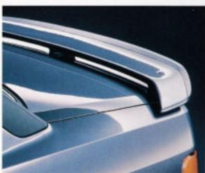
The Sierra Sapphire RS Cosworth's discreet, body-colour bootlid spoiler enhances stability by smoothing airflow over the tail. The car has an excellent 0.33 drag coefficient.
