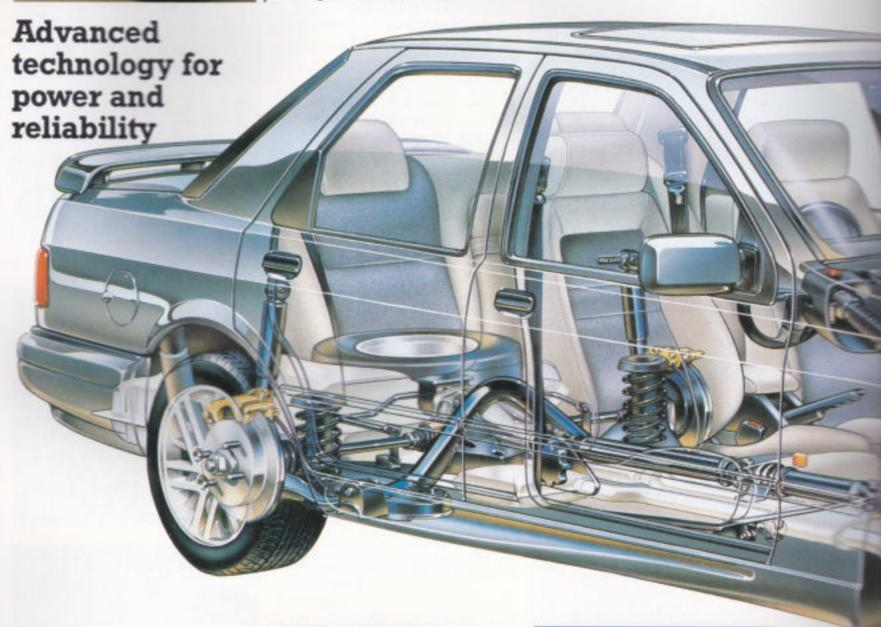
The high-torque engine's output is transmitted to the rear wheels by a close-ratio, five-speed gearbox with a light, precise shift. A limited-slip differential with a viscous coupling automatically reduces the risk of wheelspin. The coupling operates in silence, needs no maintenance, and has been proved in Ford race and rally cars.
