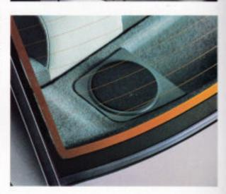
Flush channels, hidden by the door frames, carry rain water away from the roof without the need for conventional drip rails. Plastic sliders open to reveal mounting points for a roof rack.
