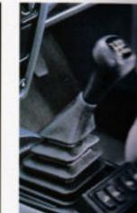
Switches for electrically operated windows are conveniently located by the five-speed gearbox's leathertrimmed lever.
