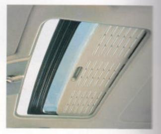
A louvred shutter shields the interior when the sun is exceptionally hot. Made of screened glass, the versatile sunroof can be slid back, or just
