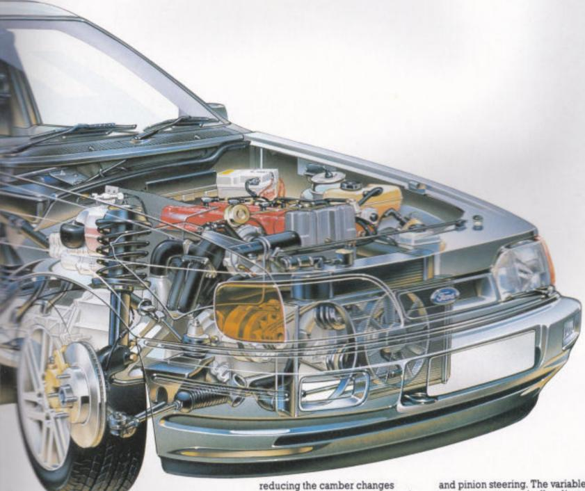
The new Ford's fully independent suspension system is engineered to combine a comfortable ride with superb grip, impeccable handling and high-speed stability. The rear layout's design keeps the tyres as 'square' to the road as possible by experienced when, for instance, the driver is forced to cut power while corning at speed. Anti-roll bars are fitted at front and rear.
